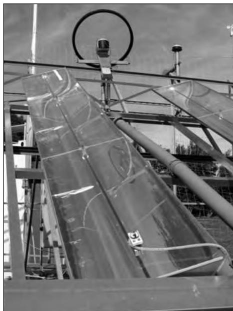
Double glazed collector with AR-glasses on an outdoor test site at Fraunhofer ISE in Germany.
